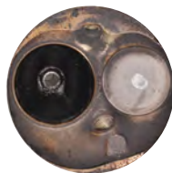
Cylinder head after one P.i. treatment.
